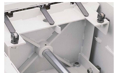
Compaction against counterplate by horizontal moving press ram
