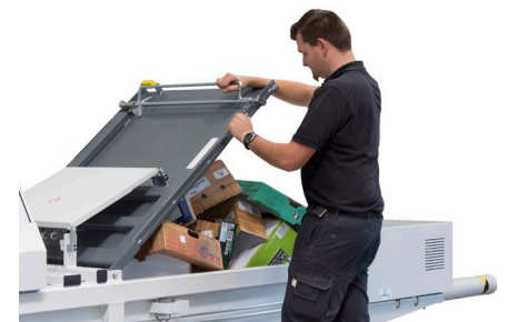
Compaction against counterplate by horizontal moving press ram
