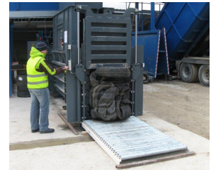
Safeguarding of the operating area with protective grid for maximum operator safety
