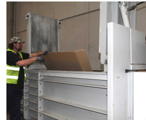
Especially large loading aperture for bulky materials
