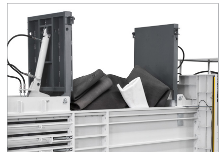
Safeguarding of the operating area with protective grid for maximum operator safety
