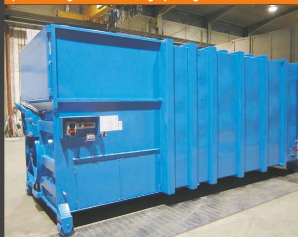
SPB LM 20 SPS in special design and with removable protective grid on the filling opening
