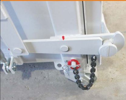
Safety chain on the discharge door (avoids uncontrolled springing open)
