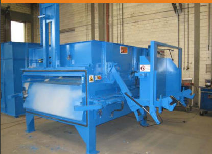
KBW 1.593 with attached bin tipper for 1,100 l waste container (MGB)
