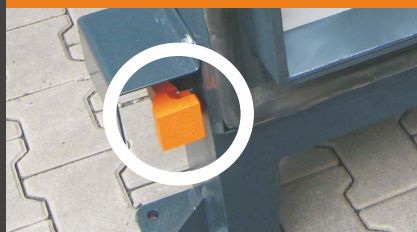
Proximity sensor (recognizes a coupled press container and enables the pressing operation)
