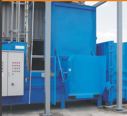
STV 1.300 with attached bin tipper and hopper with pendulum flap
