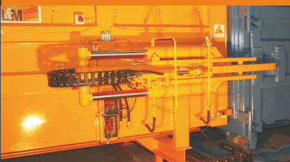
Fully automatic coupling (incl. push-of and draw-in function for the fully automatic operation with a trolley)
