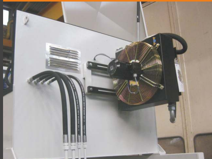
Oil cooler on external hydraulic unit
