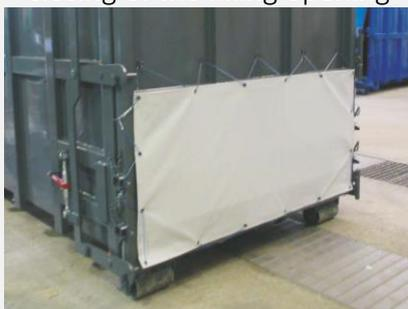
Covering hood for additional closing of the filling opening
