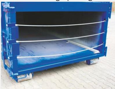
Movable tubes for closing of the filling opening
