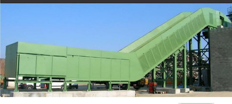
**The P400 conveyors** are fitted with a belt with folded blades, with a pitch of 400mm. This type of conveyor is used for feeding the shredder, transporting vehicles, etc.
