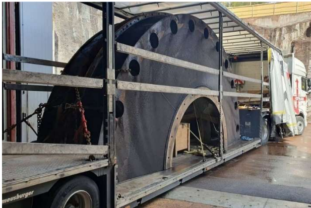
dismantled turbine cover HPP SPJUTMO, Sweden
